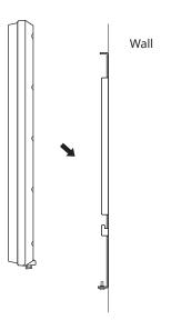
**4** Connect FaceStation F2 to the bracket by rotating the product fixing screw of FaceStation F2.
